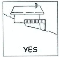
SENSITIVITY TO THE LAND: Structures should have a high degree of sensitivity to the topography of the lot and the adjacent street. Owners of neighboring lots may reject a design if the house is not a good "fit" with the lot. Structures should be designed to conform to the site, instead of changing the site to fit the structure.
